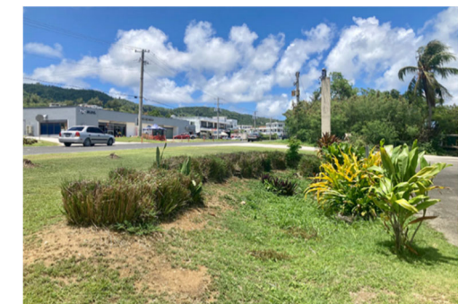
The rain garden at the NMI Museum of History and Culture in Ganagan. Rain gardens are "depressions" or "dips" that slow down water and help it drain and sink into the soil, addressing issues with erosion and potential flooding, and again, polluted waters that drains to our oceans, harming marine life. (IJA MAURIN)
